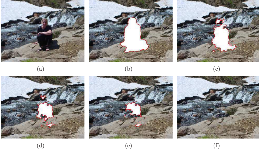
Figure 3.15: Removing large objects from photographs using Criminisi’s inpainting algorithm. (a) Original image, (b) the target region (10% of the total image area) has been blanked out, (c...e) intermediate stages of the filling process, (f) the target region has been completely filled and the selected object removed (from [30]).
