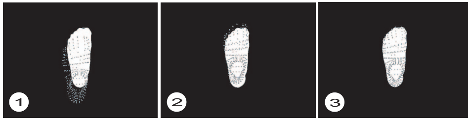
Figure 6. Silhouette images of CG foot model with the projection of sample points superimposed, during iterative process (from left to right)
