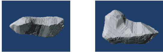
Figure 15. Reconstructed 3D model of plastic foot model by volume intersection
