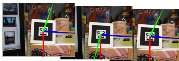
(b) Images captured in which marker plane is almost perpendicular to optical axis of a camera. It's difficult to track 3D coordinate system, especially Z axis.
