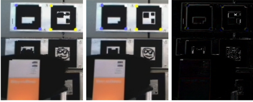
Fig. 5. Left : new view created at mid-distance between two adjacent cameras, Middle : real image, Right : difference between the real image and the computed view
