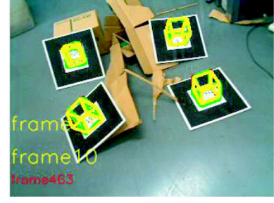
Fig. 16. The disposition of 4 markers. 4 markers are installed at different direction and uneven to each other.
