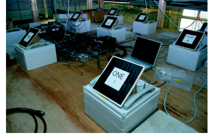
Fig. 7. AR markers installed on each modules.
