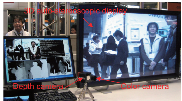
Figure 9. System for real-time 3D capturing with depth and color for auto-stereoscopic display
