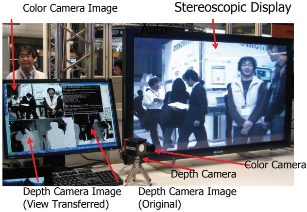
Figure 9: System for real-time 3D capturing with a depth and a color for auto-stereoscopic display.
