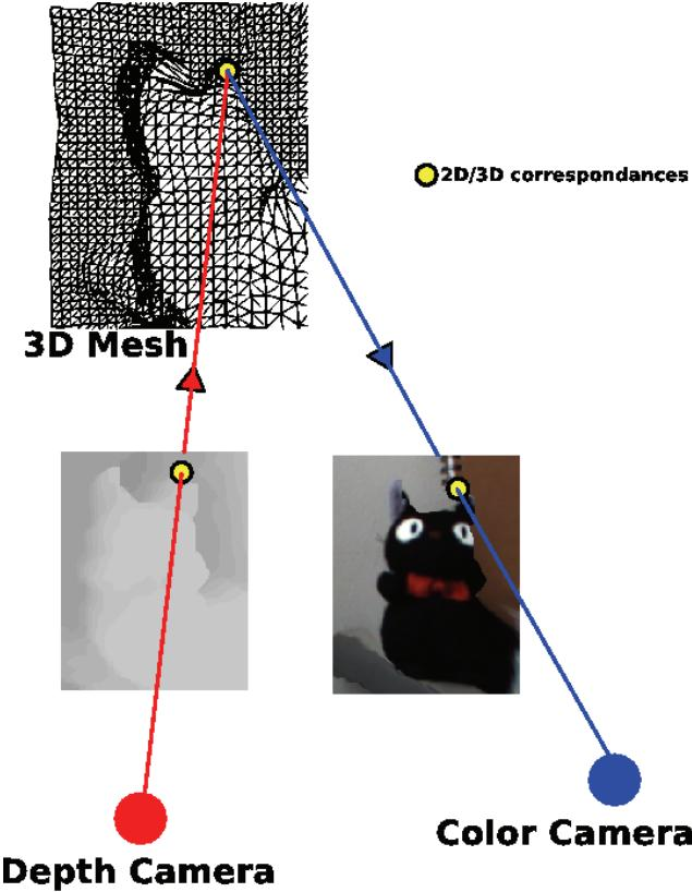
Figure 6: For each pixel of the depth-map corresponds a 3D coordinate. The depth information can be used to create a mesh and to deduce a 3D coordinate for some pixels of the color image.
