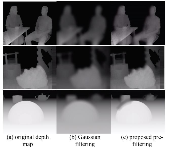
Figure 13: Examples of symmetric pre-filtering depth map with the proposed framework (from the ATTEST test sequences (top)“Interview”, (middle)“Orbi” and (bottom)“Cg”).
