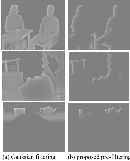
Figure 14: Error comparison between the original depth map of the pre-processed depth map (from the ATTEST test sequences (top) “Interview”, (middle) “Orbi” and (bottom) “Cg”).
