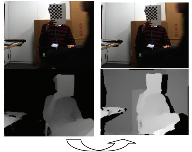
Figure 7: Example of viewpoint transfer of depth video. The depth image shown in the bottom left is transferred to bottom right, so that the viewpoint can be at the same position as the color image. (The color images on the top is the same, but shown for the comparison of the depth images.)
