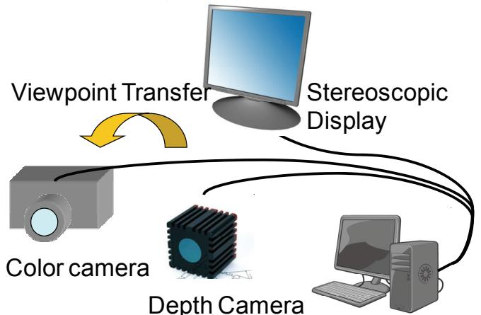
Figure 1: Depth Camera with Color camera for video capturing to display onto auto-stereoscopic display.
