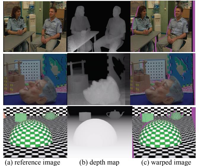
Figure 11: In magenta: newly exposed areas in the warped picture (from the ATTEST test sequences (up) "Interview", (middle) "Orbi" and (bottom) "Cg").
