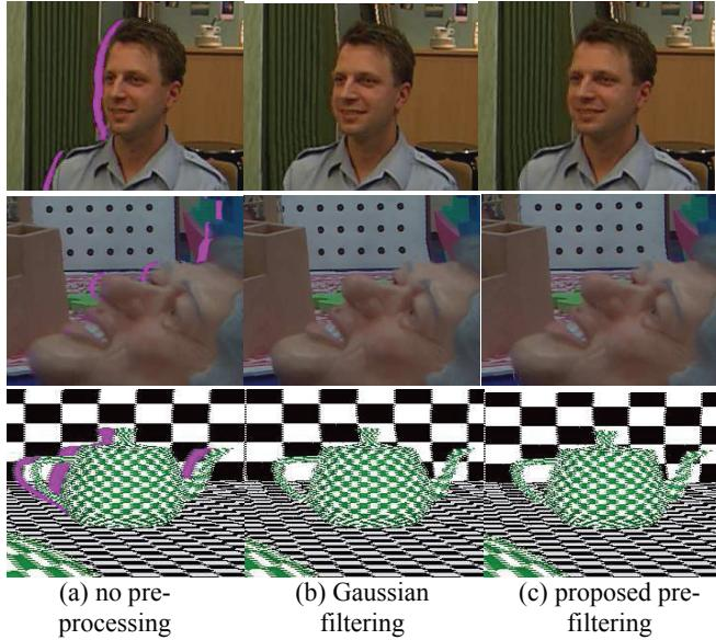
Figure 15: Warped images issue from the 3D image warping using the different symmetric pre-processed depth map (from the ATTEST test sequences (top) “Interview”, (middle) “Orbi” and (bottom) “Cg”).
