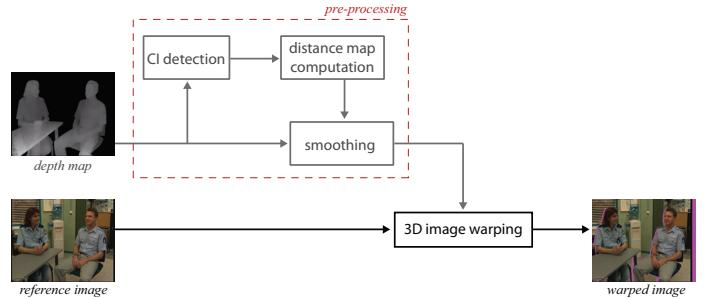
Figure 10: Pre-processing of the depth map before the 3D image warping.
