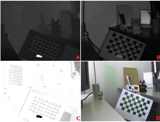
Figure 5: Four images are used for the calibration. (A) the depth map, (B) the corresponding gray scale image, (C) the confidentiality map and (D) the color Image.
