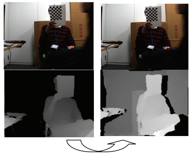
Fig.8: Example of viewpoint transfer of depth video. The depth image shown in the bottom left is transferred to bottom right, so that the viewpoint can be at the same position as the color image. (The color images on the top is the same, but shown for the comparison of the depth images.)
