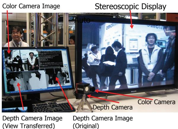
Fig9: System for real-time 3D capturing with a depth and a color for auto-stereoscopic display.
