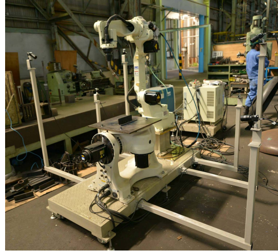
Figure 1: The multiple cameras are installed around working area of a welding robot.
