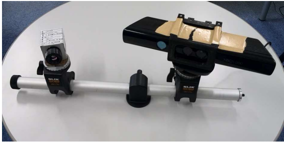
Figure 1: Our capture system is composed of the Microsoft KINECT and Optrix PI160 thermal camera.
