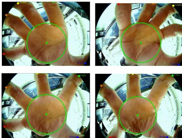
Figure 7: Finger detection when a jar is grasped in various ways
