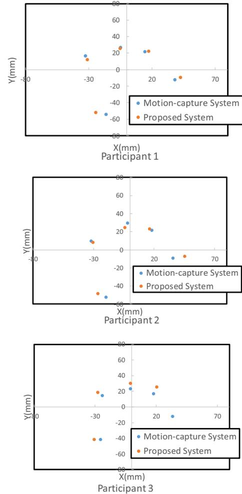
Figure 14: Comparison of fingertip positions determined via an optical motion-capture system and using the proposed system
