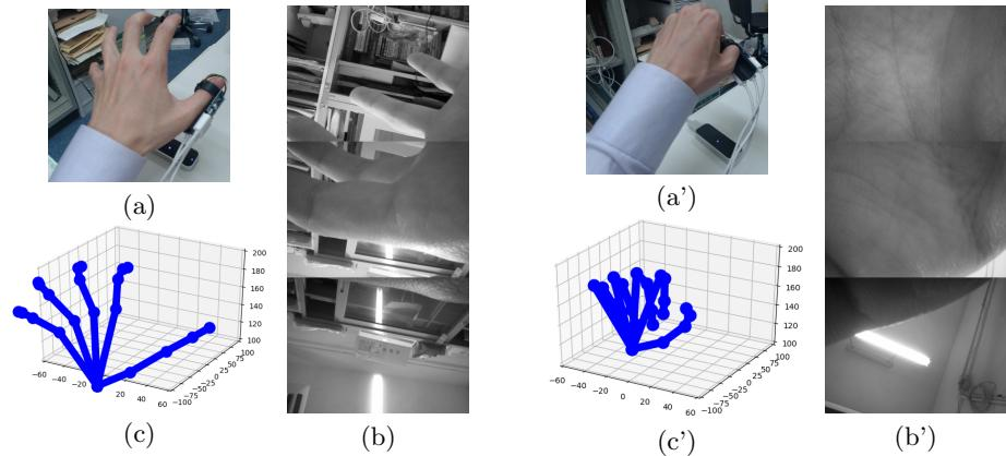
**Fig. 3.** Examples of the data collection. We used the device consisting of three cameras and the Leap Motion (a) and (a'). Three captured images are converted to grayscale, and then connected in the vertical direction to make a single image (b) and (b'). The Leap Motion provides the 3D positions of the hand keypoints (c) and (c').
