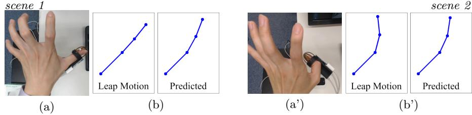
**Fig. 5.** Two specific examples of testing, *scene 1* and *scene 2*. the hand states (a) and (a'), and the states of the thumb are reconstructed by  $\theta_1$  and  $\theta_2$  (b) and (b'). The left of (b) and (b') was created based on  $\theta_1$  and  $\theta_2$  acquired by the Leap Motion, and the right was created based on the predicted  $\theta_1$  and  $\theta_2$ . Note that other parameters (e.g., finger length) are appropriate values because only angles were estimated.
