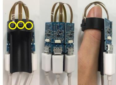
**Fig. 1.** The thumb tip wearable device we developed. Three cameras (left, circled) and their driving circuits are fixed to the device (center). The device can be attached to the thumb as shown on the right.
