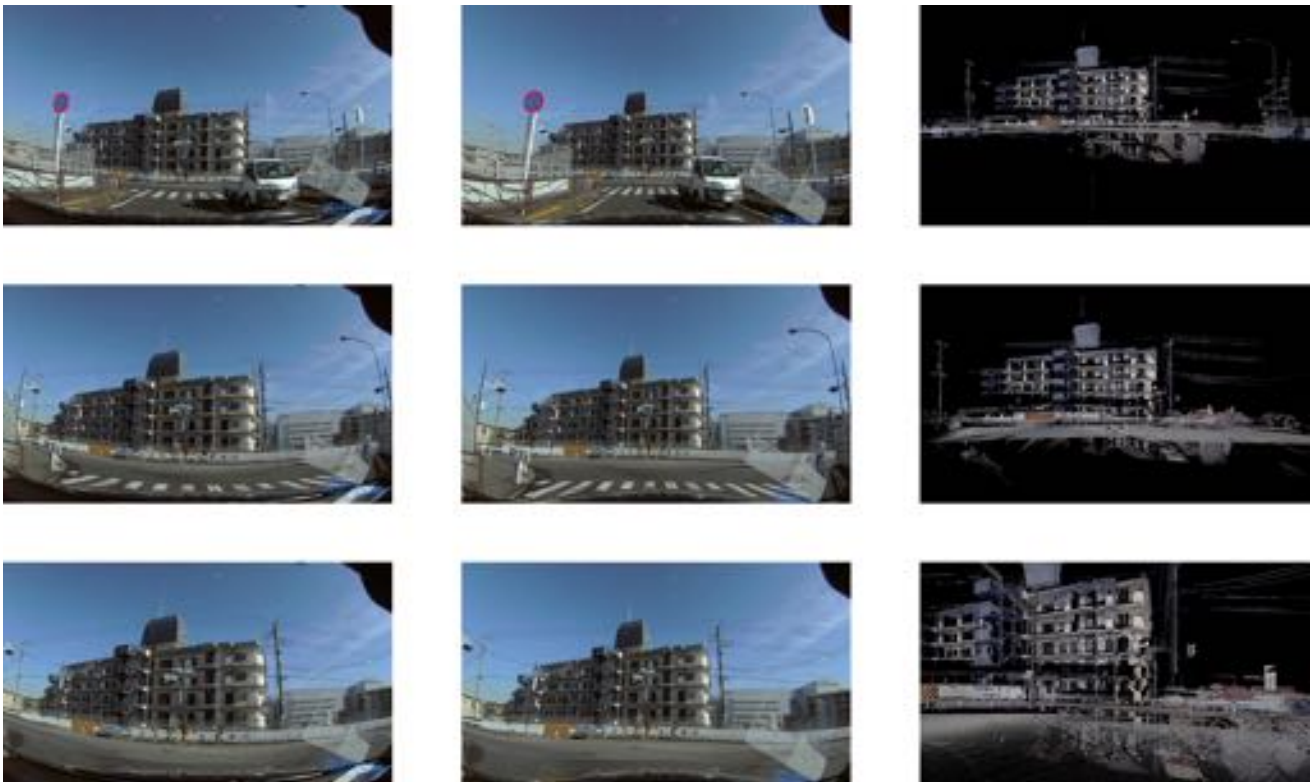
Figure 10. Left: Original drive recorder images, Center: Image with distortion removed, Right: Images generated using the estimated position and orientation.
