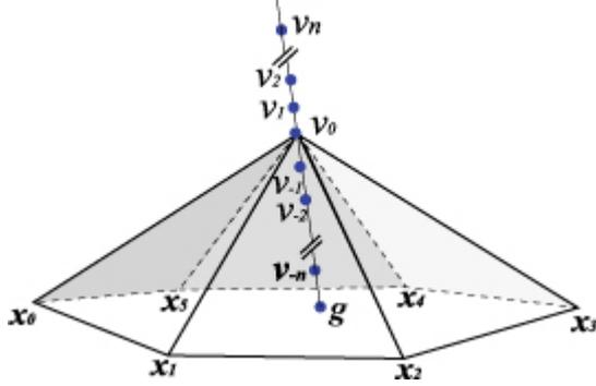
**Figure 1. Deform of vertex: Moving candidate points are defined on a line  $v_0$  to  $g$ .**
