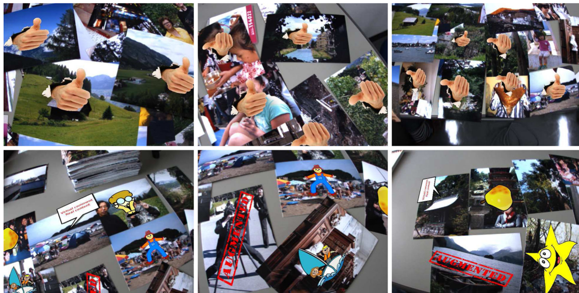
Fig. 11 Augmenting multiple objects simultaneously. Our system retrieves, tracks, and augments the pictures lying on the desk. On the first row , all the objects are augmented with the same virtual content.
