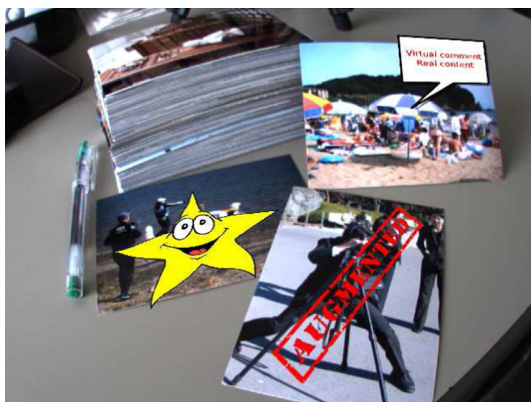
Fig. 1 To produce this result, our system detects, identifies, and tracks the photographs visible on the input video stream. Each picture is augmented with its corresponding virtual element, precisely registered. The stack of pictures visible on this image contains about 300 images. Our system can recognize all of them. Users can also augment new objects by simply showing them to the camera and clicking. Tracking and augmentation start right away
